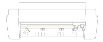
5. Use rubbing alcohol or other adhesive remover on a cotton swab or paper towel to wipe off any residual adhesive or debris from the cutting strip area.
