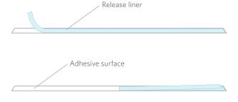
7. Adhere the cutting strip starting from the left side of the machine (adhesive side down) along the front edge of the groove. Make sure to leave a small gap between the cutting strip and the left edge of the groove.
