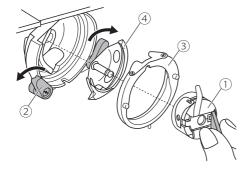
Remove the bobbin case. Snap the two hook retaining arms outwards. Remove the hook race cover and the hook and clean withe a soft cloth.
