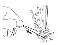
Pull both threads to the back under the presser foot.
