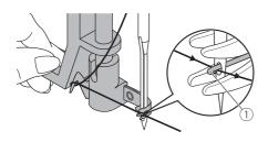
Hold the thread loosely and release the lever slowly. The hook turns and passes the thread through the needle eye forming a loop.
