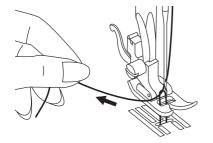
Gently pull on the upper thread to bring the bobbin thread up through the needle plate hole. The bobbin thread will come up in a loop.
