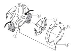
Replace the hook. Attach the hook race cover making sure the bottom pin fits into the notch. Snap back the two hook retaining arms. Insert the bobbin case and bobbin and replace the stitch plate.
