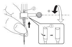
When inserting a new needle, keep the flat side of the shaft to the back.
